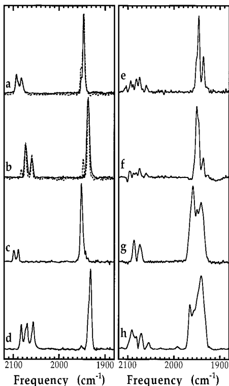
Figure 2. FT-IR spectra of hydrogenase films in different states and from different sources. Left: D. gigas enzyme in (a) as-isolated, before (—) and after (---) L-edge experiment, (b) H 2 -reduced, before (—) and after (---) L-edge experiment, (c) dithionite-reduced, and (d) CO-inhibited states. Right: (e) as-isolated D. baculatus , (f) H 2 -reduced D. baculatus , (g) as-isolated P. furiosus , and (h) H 2 -reduced P. furiosus enzymes.
